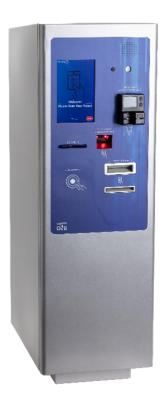
The operating temperature can range between -40° and 130° F and 10-95% non-condensing humidity with heater kit. The device has easy-to-use side and front access panels with a hinged door that is key-accessible by authorized technicians. Each device is typically mounted to a five- or six-inch concrete curb with four internal mounting bolts.
