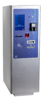
The operating temperature can range between -40° and 130° F and 10-95% non-condensing humidity with heater kit. The device has easy-to-use side and front access panels with a hinged door that is key-accessible by authorized technicians. Each device is typically mounted to a five- or six-inch concrete curb with four internal mounting bolts.
